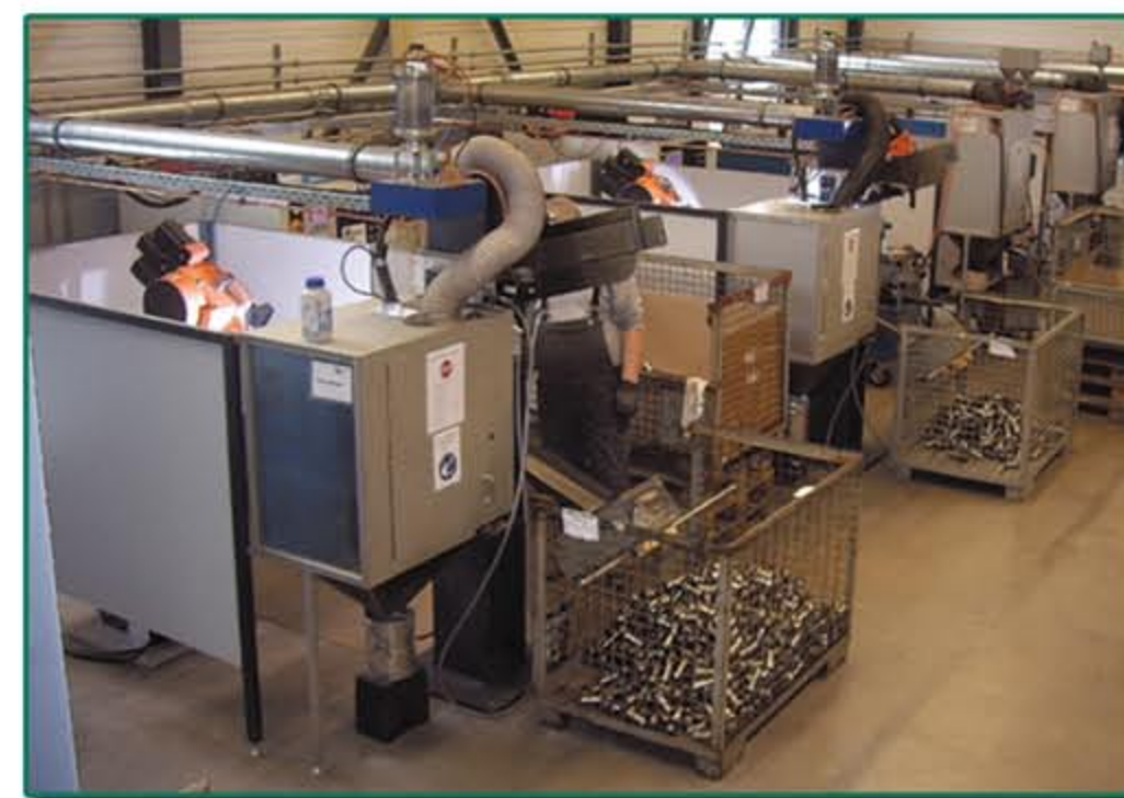
Panzer Splitt hardfacing facility
